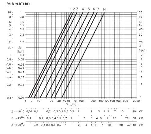
Capacities at  $X_p = 2K$  with Danfoss radiator thermostat RA 2000 are measured without radiator and connection fittings.
